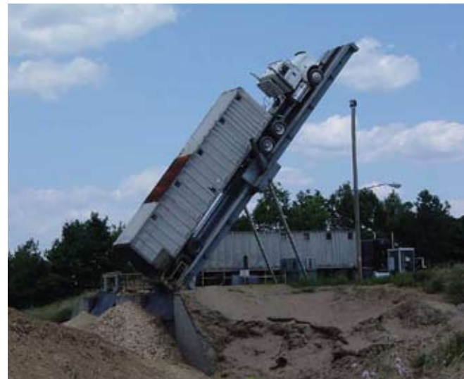
At Pittsylvania Power Station in Hurt, Virginia, leftovers from sawmills, logging operations, and paper mills provide electricity for about 20,000 homes. An estimated 3,300 tons of wood waste is unloaded each day at the plant, which translates to about 150 truckloads.
